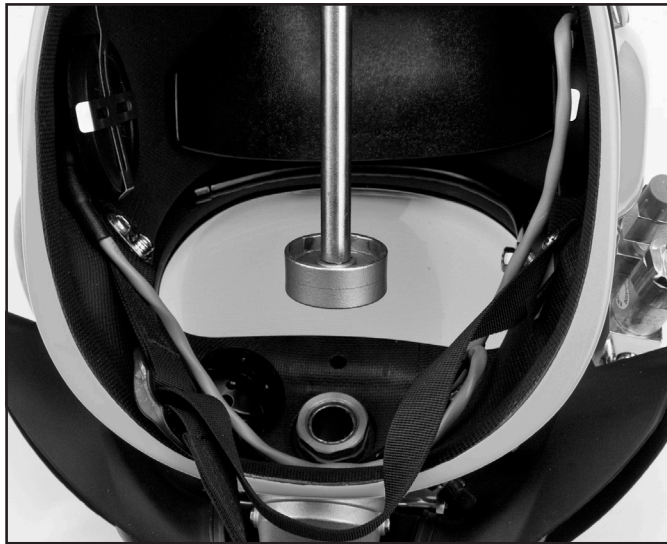
The regulator mount nut must be loosened with a wrench.
