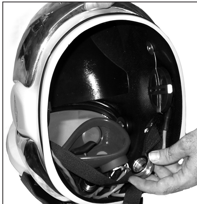
Remove the mount nut from the regulator.
