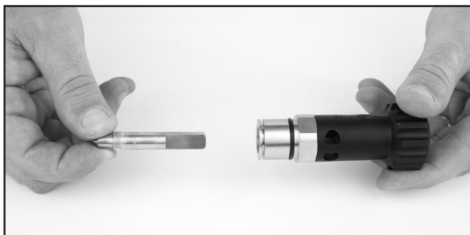
Lubricate threads on adjustment shaft with Christo-Lube® and insert into flex knob
