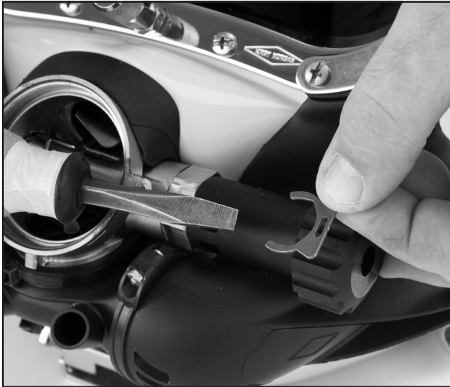
The lock clip must be removed to service the internal O-rings in the regulator.
