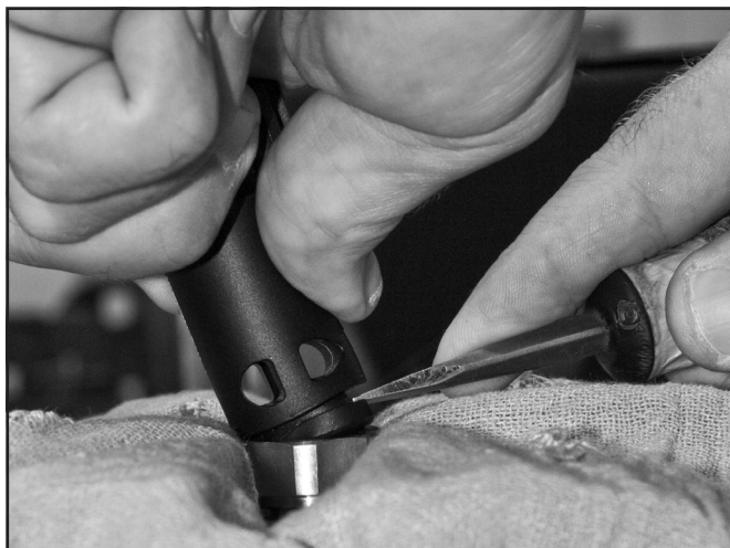
Place packing nut in vise and use a slotted screwdriver to insert flex knob
