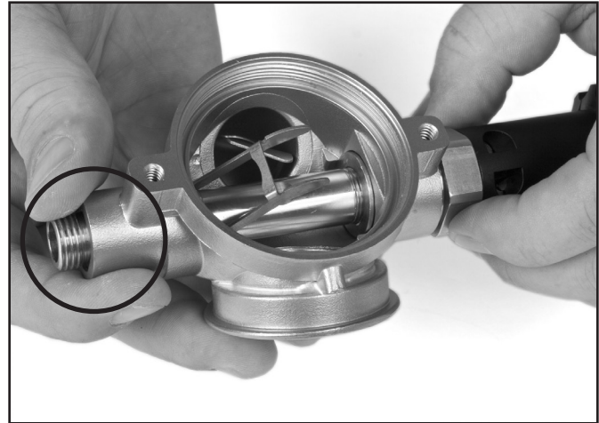
The end of the threads on the main tube should be flush with the opening of the tube on the side of the regulator body.
