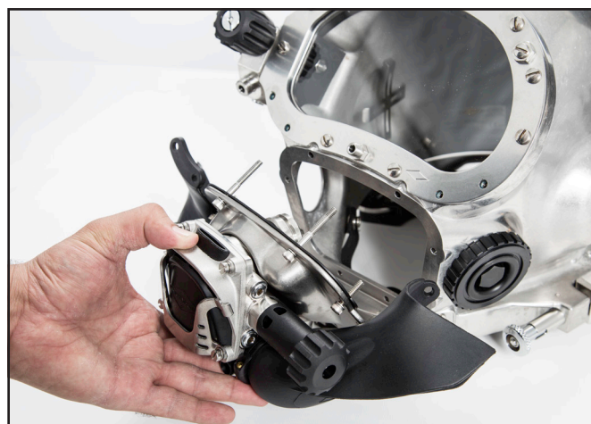
Separate the pod/regulator assembly from the helmet shell.
