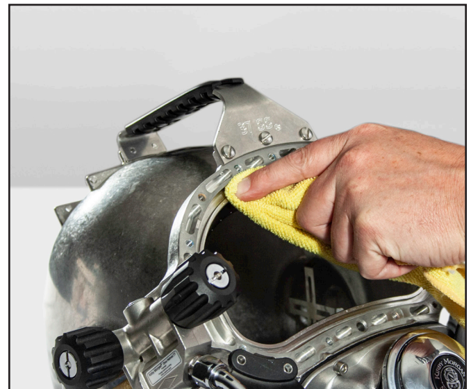
Clean the O-ring groove prior to replacing the face port O-ring.
