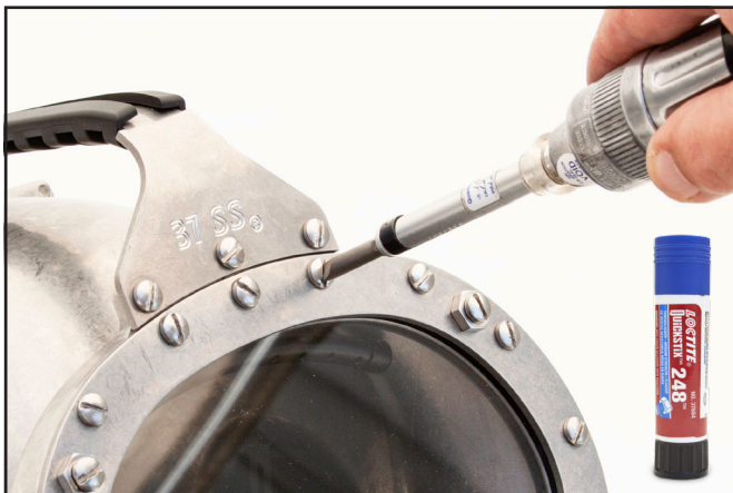
Always use a torque screwdriver to check the tension of the port retainer screws.
